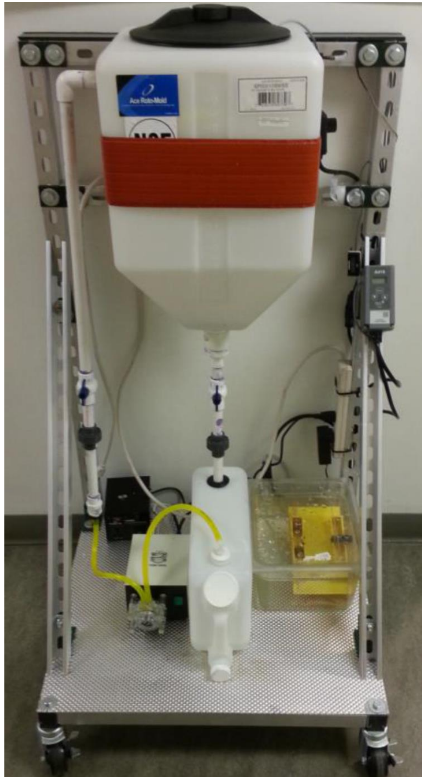
Figure E.6: Photograph of fully-constructed 10-gallon pilot-scale HS-AD system.
